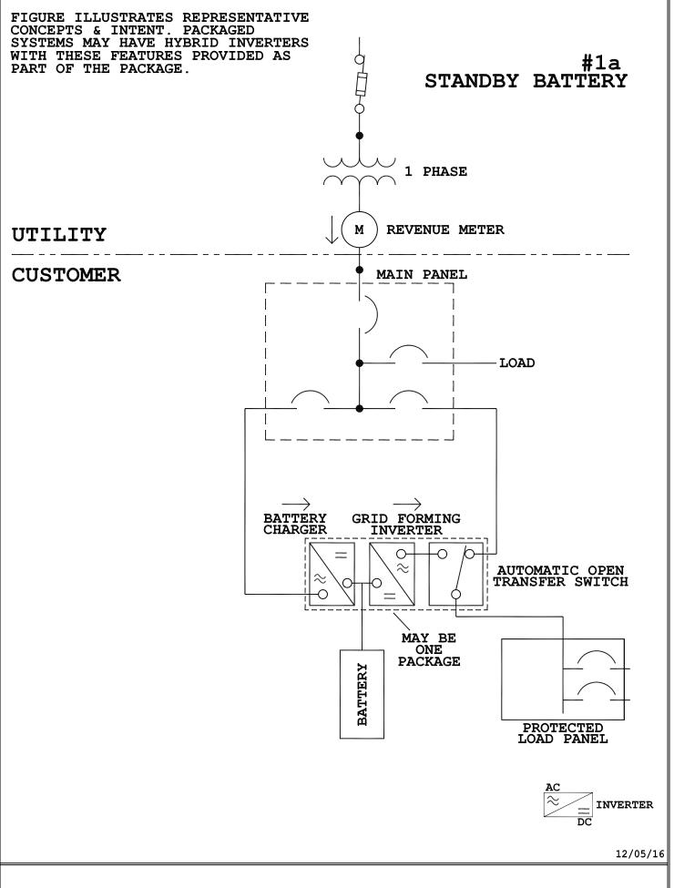
FIGURE ILLUSTRATES REPRESENTATIVE CONCEPTS & INTENT. PACKAGED SYSTEMS MAY HAVE HYBRID INVERTERS WITH THESE FEATURES PROVIDED AS PART OF THE PACKAGE.
